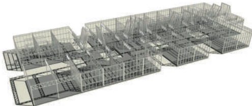
2. Trusses and skylight structure
